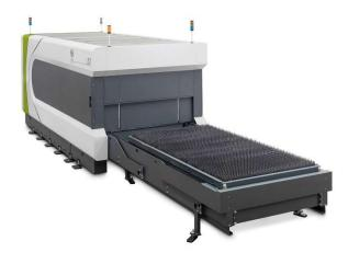
The cutting area has been designed to protect the bellows from the glowing sparks thrown in all directions, especially during the initial piercing of the material. With access from the short side, the entire machine remains completely enclosed for safety reasons related to the fibre laser source. The cutting process can be viewed on a camera whose image is visible on the operator console, via an additional external monitor and also remotely. **Cutting quality**
